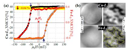
**Fig.1**: (a) Element-selective XMCD hysteresis loops of a [1.8 nm Pt/0.6 nm Co]<sub>8</sub>/10 nm FeMn system recorded in transmission geometry. XMCD data are normalized to their corresponding absorption  $L_3$  peaks. (b) Magnetic domain images of the FM layer (top) and the uncompensated AFM moments (bottom) at selected applied fields. FOV=1.8 µm. The images are retrieved from the Fourier transform of magnetic holograms acquired at the Co- $L_3$  and Fe- $L_3$  absorption edges, respectively.
